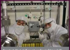
anotech West staff members Derek Ditmer (left) nd Stacy Coil with their new tool interlock box. A SB line leads to the front of a spin coater in the hotolithography bay and makes the tool available by nabling the vacuum hold-down for the spin chuck.
