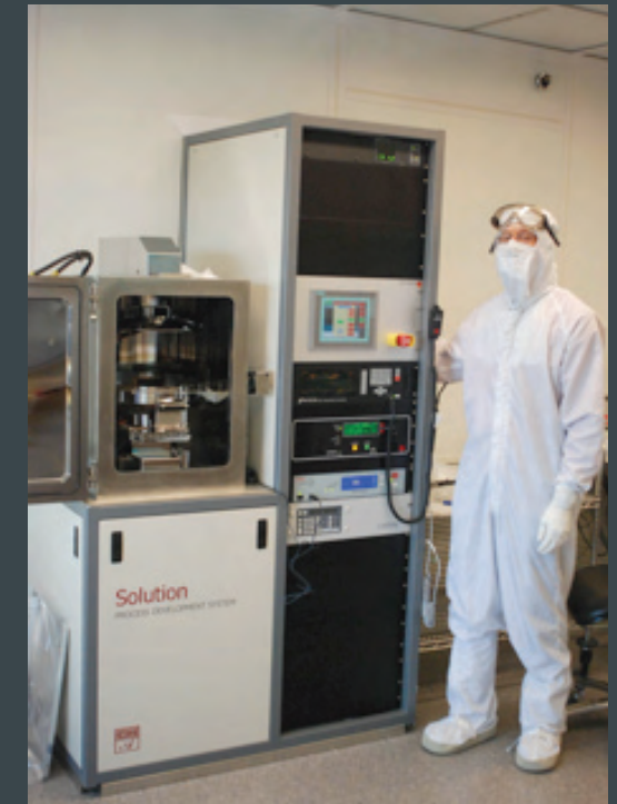
Nanotech West Lab staff member Paul Steffen and the new 6 pocket CHA SOLUTION™ System electron gun evaporation system in Bay 4 of the cleanroom.
