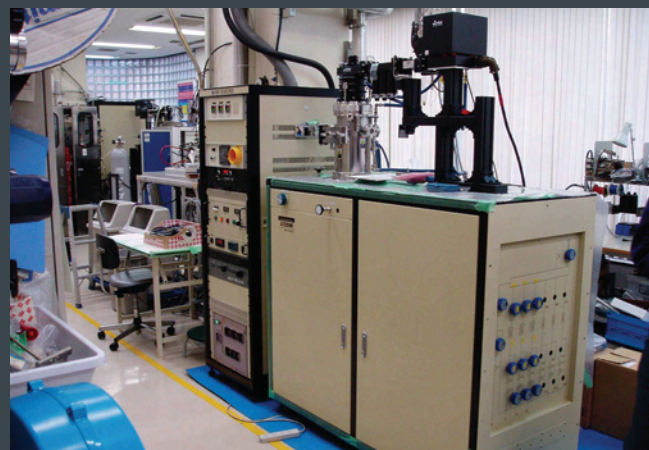
Seki Technotron Corp. AX5200M 1.5kW Microwave-Plasma Enhanced-Chemical Vapor Deposition system
