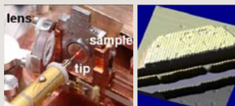
Figure 4. (left) Picture of custom STM stage. (right) STM image of an island of \text{C}_{60} on \text{Ag}(100) . We are studying tip-enhanced photo-polymerization of \text{C}_{60} within such islands.
