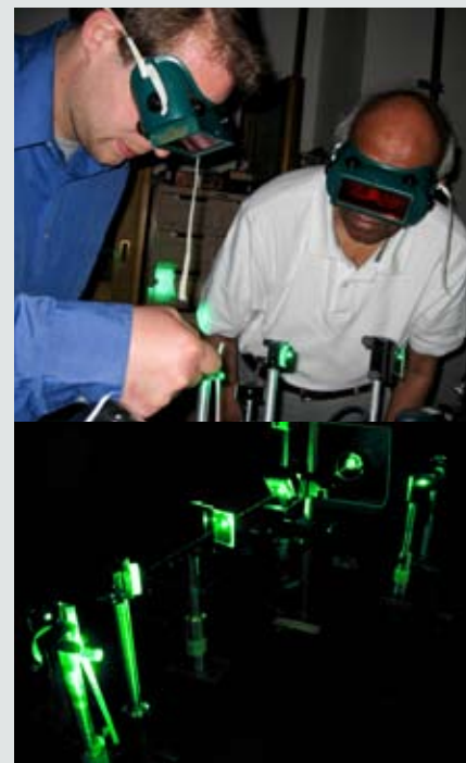
Sheldon Bailey, graduate student in Physics, and Professor R. Sooryakumar adjusting optics for the detection of high frequency acoustic waves.
