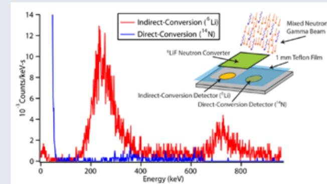
Figure 1: Neutron detection spectra with schematic from Prof. Cao's research
