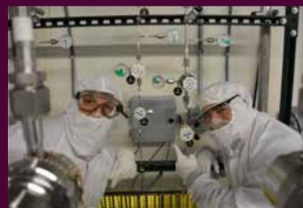
Nanotech West staff members Derek Ditmer (left) and Stacy Coil with their new tool interlock box. A USB line leads to the front of a spin coater in the photolithography bay and makes the tool available by enabling the vacuum hold-down for the spin chuck.
